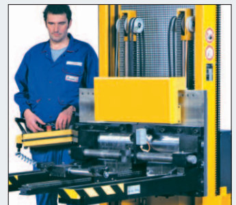
Hydraulically driven horizontal traverse of the entire carrying fork
