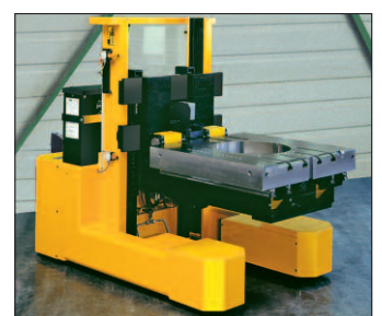
DILOS TRUCK 40 with special open chassis for lowering a special carrying fork to floor level
