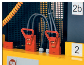
Plug connectors for quick attachment and disconnection of the batteries
