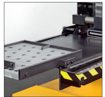
Accessories: Integrated board with transport balls for changing small modular dies
