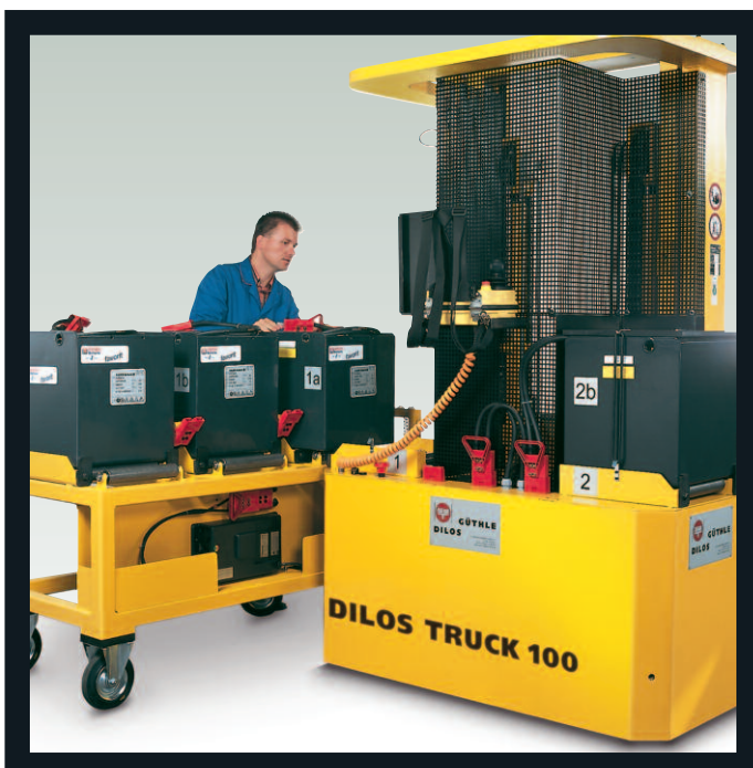
DILOS battery-changing trolley with charger for shift operation
