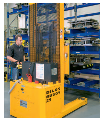
DILOS BUGGY 25 SPECIAL with operating panel and traversing fork sled
