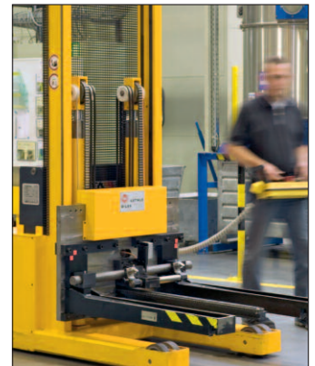
For safety reasons, the loaded fork is lowered to chassis level for travel. Control turns automatically to slow speed when fork is raised.
