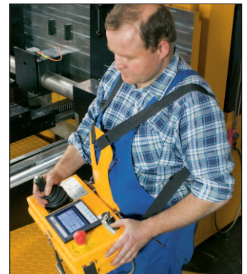
With the joystick, the operator can control all functions delicately. The display shows the attitude of the wheels, among other information.
