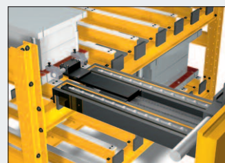
DILOS double rack with slide support beams, usable from both sides. A DILOS TRUCK 40 is docked in front of one of the racks (height for standard lift range) and is removing a die
