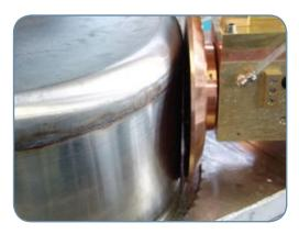
CEMSA manufacture automatic seam welding solutions, like the "ROBOSEAM", for high quality welding, in a cooling water bath, delicate materials sensible at the overheating (stainless steel in different grades), on a working table with a copper plate of variable sizes up to cm 1000 x 2000 mm
