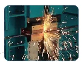
By this EVO control package installed on the STI welders, customers are able to program in details all variables and to detect and see in real time the applied forces, heat and speed variations, as well as to save data for certifications of the products.
